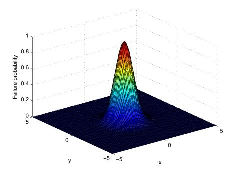
Figure 1: An example of spatial failure probability distribution that occurs in (0,0), where a component fails with a probability that corresponds to its distance from the failure epicenter.
