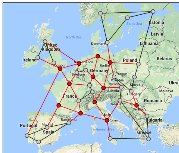
Figure 1: Cost266 network visualization over a map. Red nodes represent removed nodes (in this case the 30% of nodes).
