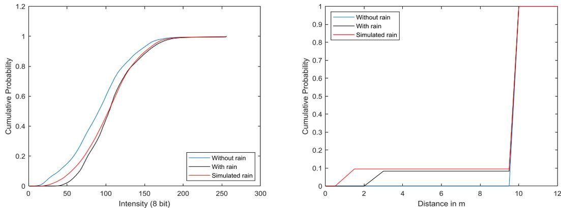
Figure 2: Cumulative histograms of camera images (left) and point clouds (right) including no, real, and simulated rain conditions. The blue curve represents the condition without rain, the black curve the real rain condition, and the red curve the simulated rain condition. Static scenario: Target vehicle is placed at a distance of 10 m and is measured by camera, lidar, and radar sensors.
