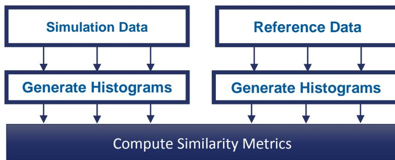
Figure 1: Histogram-based approach for validating the simulated output of each surround sensor in the same way.
